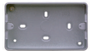
K8902 ALM 4 x 20mm & 4 x 25mm Knockouts 46mm Deep Box
